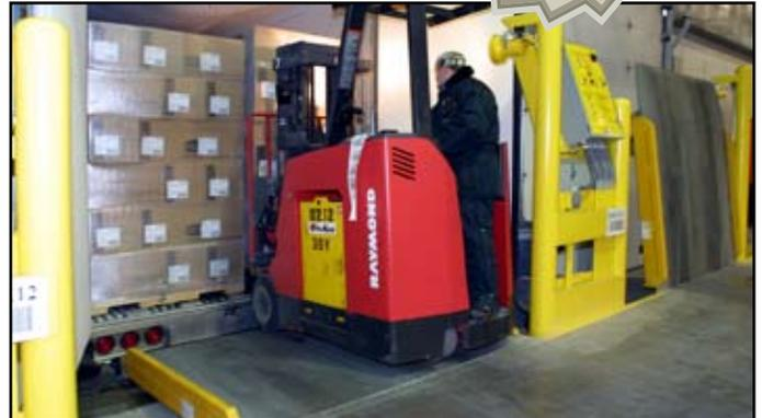
Full and independent control of dock leveler lip and dock functions permits easy "end loading" when trailers are fully loaded to the rear of trailer.
