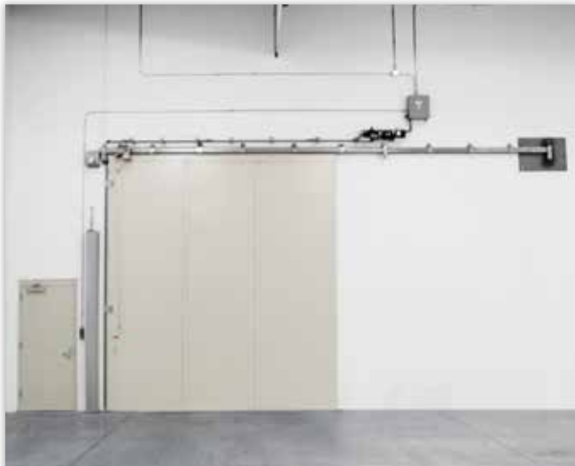
Saino Model 1000 with 1900 operator with explosion proof motor & intrinsically control mounted in NEMA-12 Control Box.
